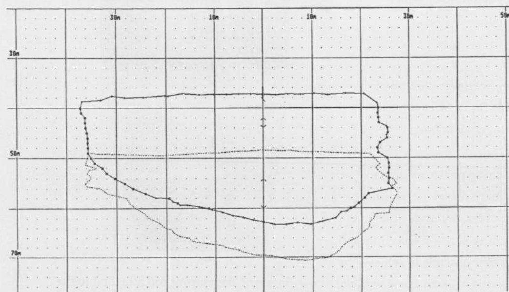
Figure 6. Good control of cavern-shape during the main leaching phase with vertical walls and a flat roof (1995 - 97)
